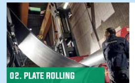
Try to roll a small sheet of metal into a perfect circle. It isn't that easy to get it just right. Now, imagine rolling a massive sheet of steel into a perfect circle of up to ten meters in diameter, where millimeter precision is essential. Quite a task, right.
